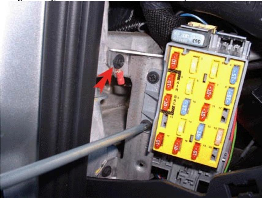
Soldering: Now the Green and the Red wires (from the TT). The Green was soldered to the back of the fuse block at # 9 (just make sure it is between the tan w/green strip and the solid green). Now the Red wire ( from the Turbo Timer) is connected to the # 14 spot.
