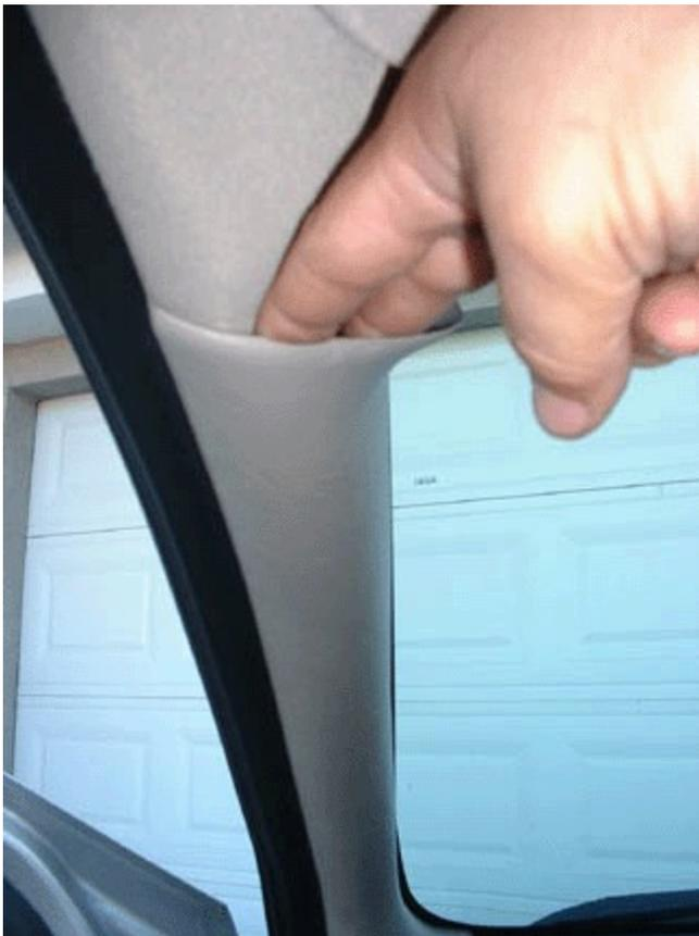
You will need to place your index and middle finger along the roof going under the top of the side pillar then gently pull towards the seats. There are two metal clips per side/pillar (the top one might break if it does this isn't a major problem the pillar will still stay in place when put back).
