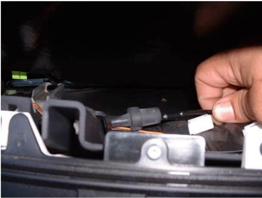
Now before you try to pull the dash out of the car you will need to unplug the boost gauge and the light for the boost gauge. These are going to be right in front of you as you are sitting in the drivers seat. The vacuum line just needs to be pulled to separate and the light wire has a clip that you need to press on to separate.
